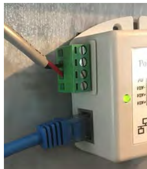
Power Connection & Internet RJ45 Input
