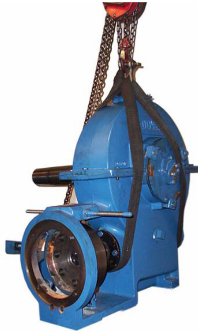
Figure 48 - Gear Case with Hoisting and Rigging
