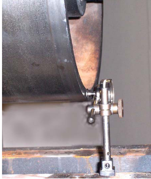
Figure 34 - Dial Indicator on Brake Hub
