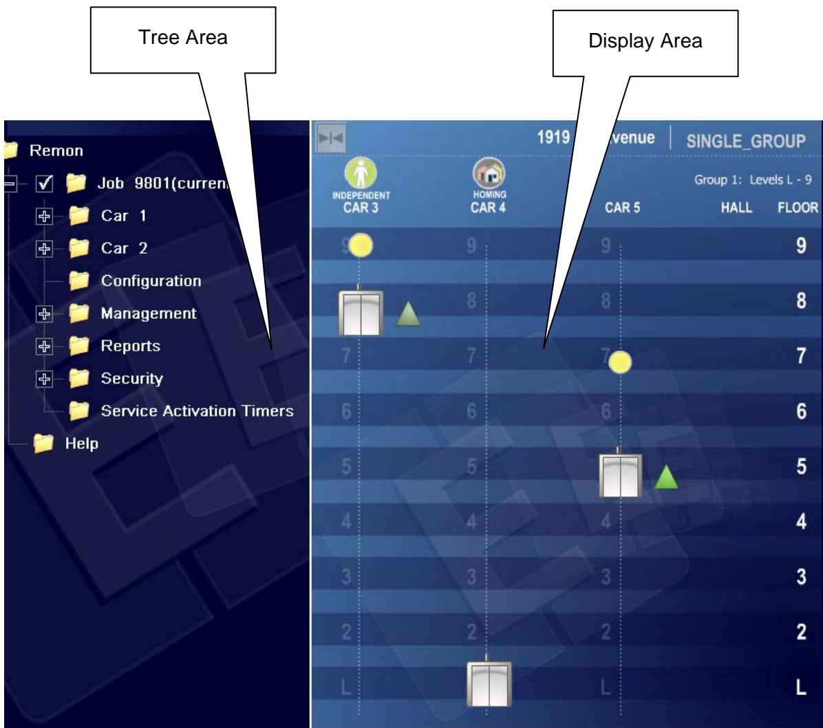
Figure 5: Main Screen, Client Application Software
